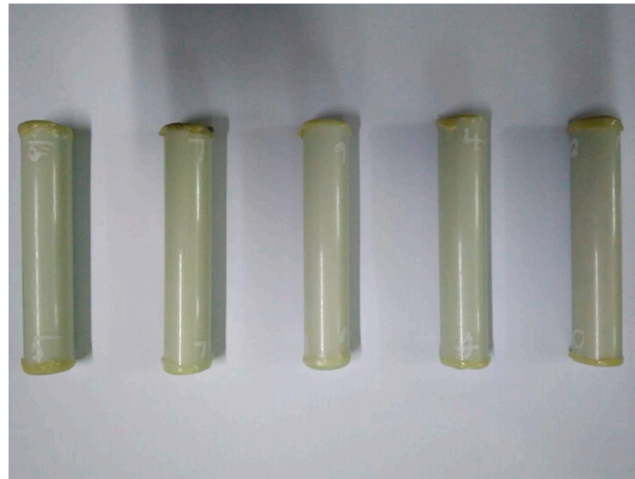
Figure 3. Rod specimens with the length of 100 mm for water absorption. Note, the ends were capped with an epoxy adhesive.
