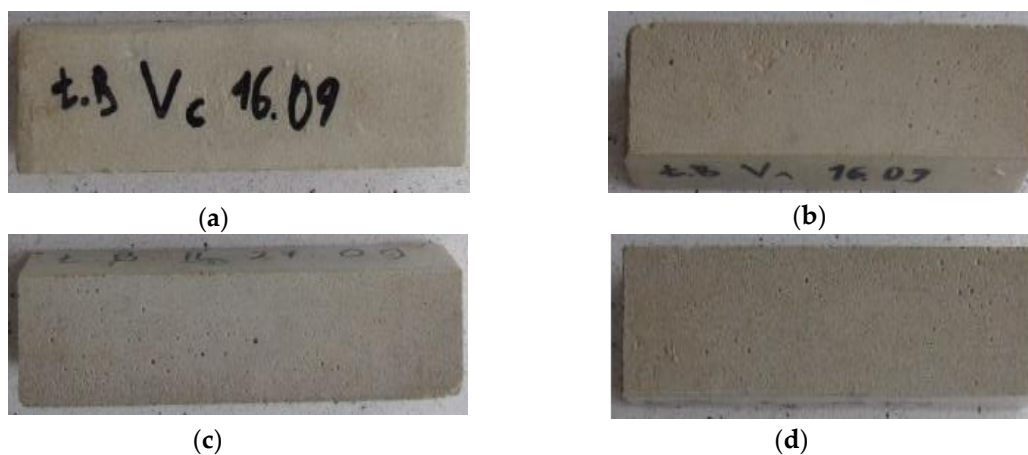
Figure 7. Condition of representative samples before the frost resistance test: (a) SM; (b) CM0.5; (c) CM1; (d) CM1.5.
