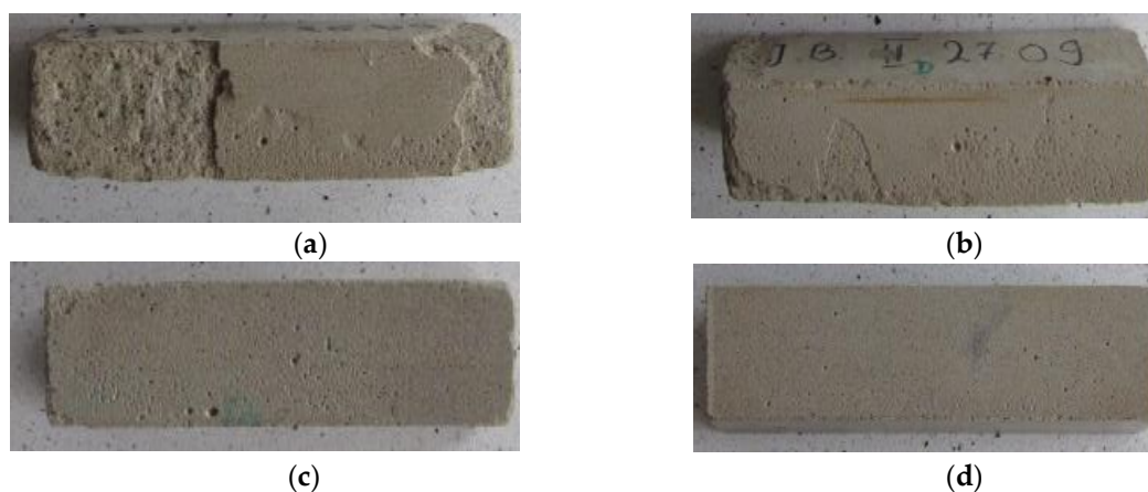
Figure 8. Condition of representative samples after the frost resistance test along with the mean mass loss: (a) SM; (b) CM0.5; (c) CM1; (d) CM1.5.
