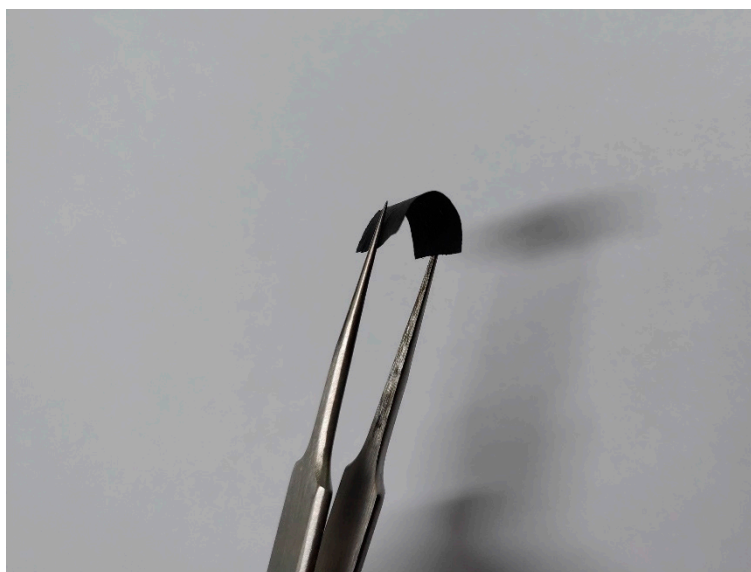
Figure S4. Photograph of composite film (polymer/SWCNTs with a mass ratio of 50/50) in bending state.
