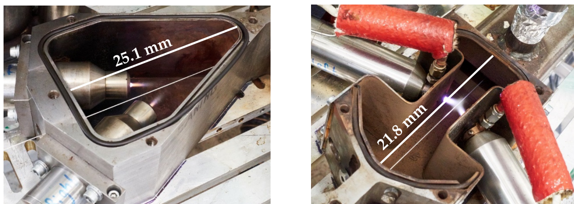
Figure 1. Left: decontamination chamber; right: plasma coating chamber.
