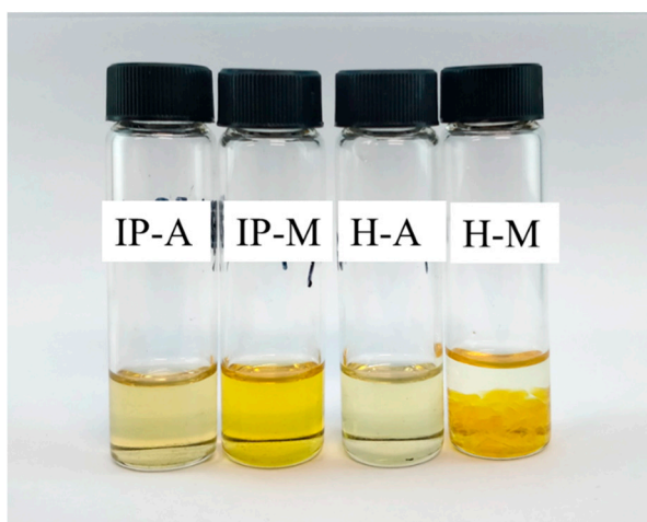
Figure S5. Different solubilities of the four polyureas in DMF after 24 h.
