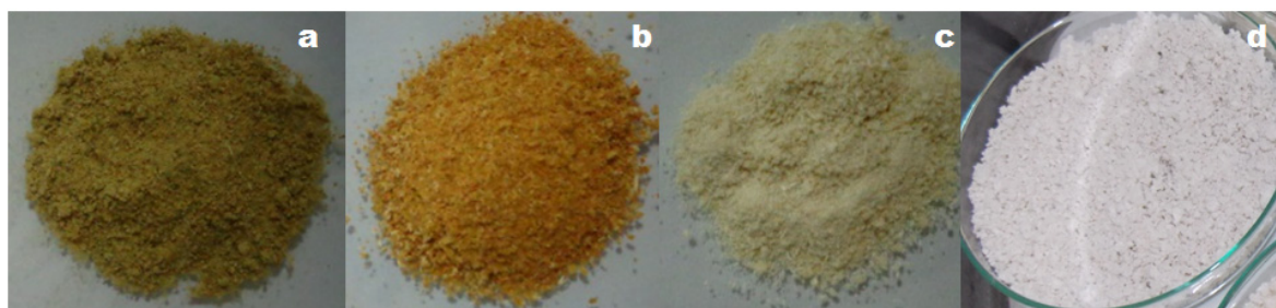
Figure 1. Technological processing of Opuntia ficus-indica L. Miller for cellulose extraction. (a) powdered plant, (b) powdered plant free of impurities, (c) holocellulose and (d) cellulose.
