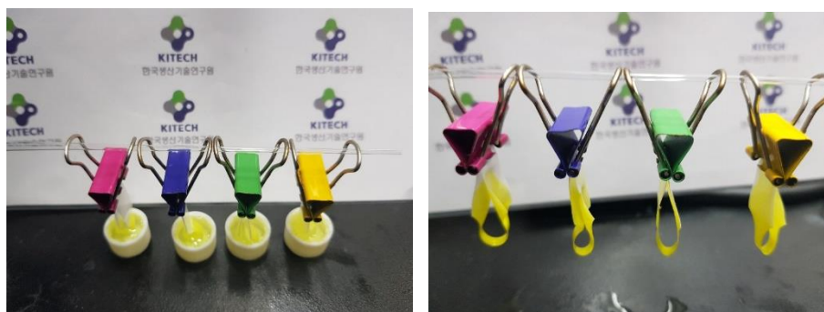
Figure S5. Sample preparation for measuring the mechanical property changes of UiO-66/DSPD composite films after MPO decomposition test.
