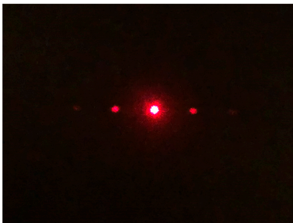
Figure 5. Far-field diffraction image of the output beam transmitted through the periodic structure processed 150 μm underneath the surface, with 20 μm inter-line spacing and 1 nJ pulse energy at 0.50 mm/s.
