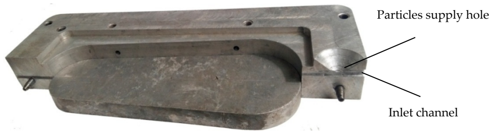
Figure 5. Mold for making soles with recycled polymer waste particles.
