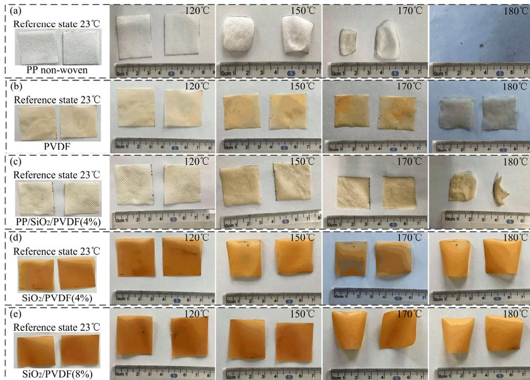
**Figure 5.** Thermal shrinkage properties of the film: (a) thermal shrinkage of PP non-woven materials under different heat treatment temperature; (b) PVDF; (c) PP/SiO<sub>2</sub>/PVDF (4%); (d) SiO<sub>2</sub>/PVDF (4%) and (e) SiO<sub>2</sub>/PVDF (8%).
