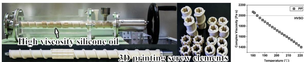
Figure 8. Visualization test stand: general view of extruder with visualization feature used in the experiments.
