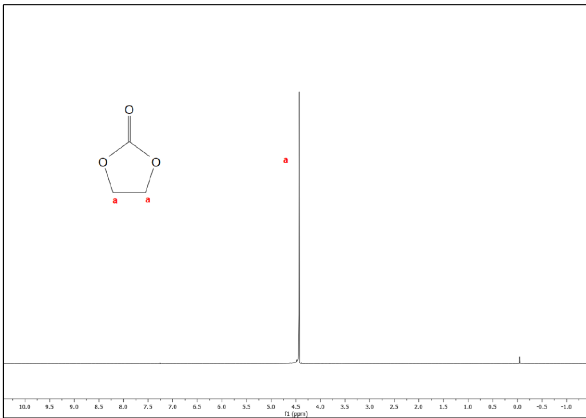
Figure S11. 1 H NMR (400 MHz, CDCl 3 - high concentration, solvent signal not visible) spectrum of the product of reaction 14 (Tab.1) – ethylene carbonate
