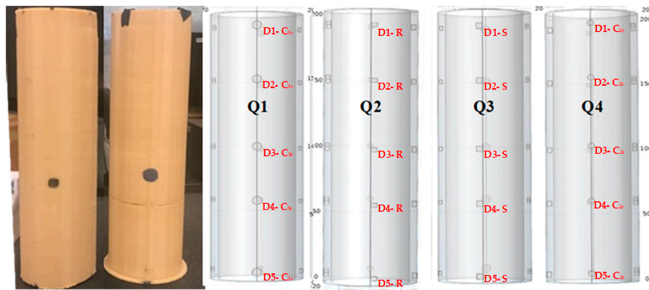
Figure 2. The 3D-printed coupons for the cylinder samples and the COMSOL® model with the four different quadrants.
