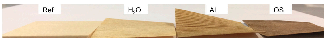
Figure 2. Representative photographs of single veneers in untreated condition (Ref), densified after soaking with water (H 2 O), densified after alkali-delignification (AL), and densified after organosolv delignification (OS).
