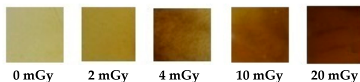
Figure 2. Visual color change of PVA/NBT films before and after exposure to varying doses of X-radiations.
