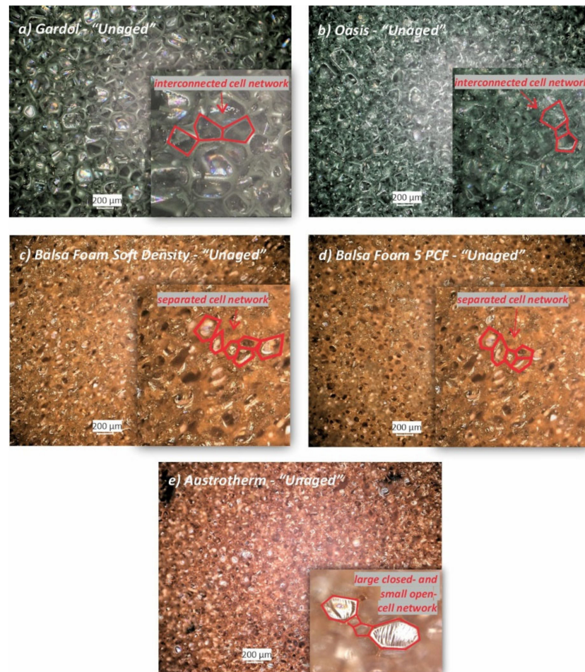
Figure 2. Photomicrographs of the “Unaged” phenol formaldehyde (PF) foams (a–e) investigated by a digital microscope with reflected light.
