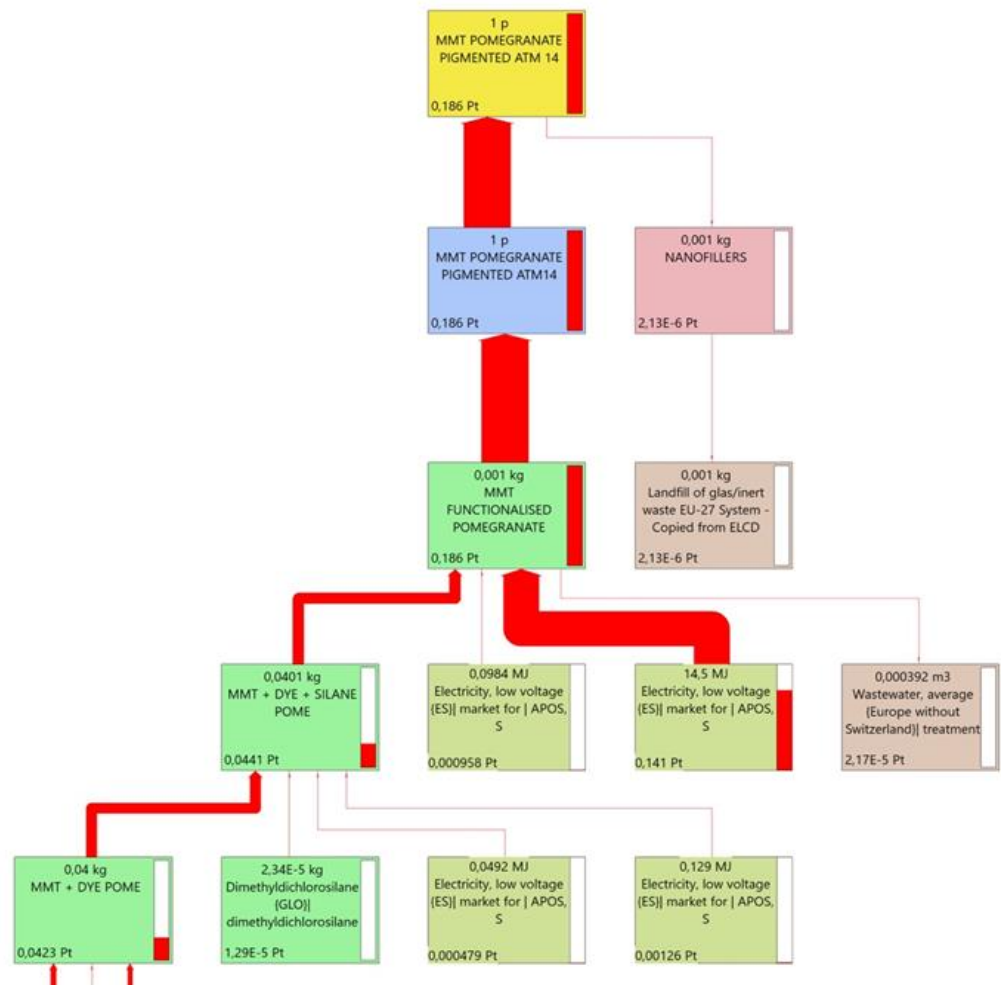
Figure S1. MMT-based PDNPs process tree and details of the three sections: pomegranate dye extraction (a), MMT functionalization with surfactant and mordant (b) and nanohybrid preparation (c).
