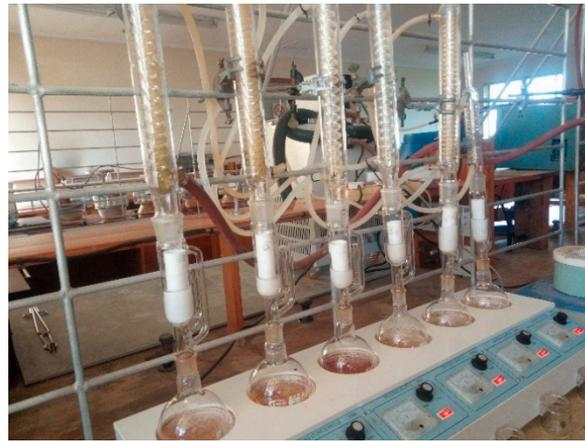
Figure 5. Soxhlet extraction setup for biomass compositional analysis.
