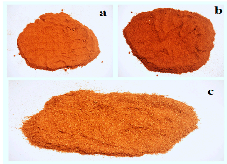
Figure 1. Saw-dust of weight densities (a) 200 kg/m 3 (b) 250 kg/m 3 and (c) 300 kg/m 3 .
