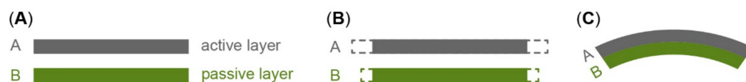
Figure 7. (A) Bimetal consists of two layers of metal with different rates of thermal expansion; (B) these metals, when heated, expand differently; (C) such layers are permanently linked to each other. As the passive layer limits the active layer, the bimetal compound follows a deflection curve when heated. Source: adapted from [16].
