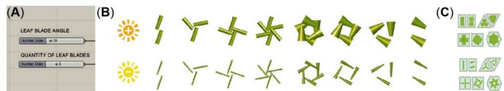
Figure 10. Parametric leaf-blade system: (A) parameters for replicating the modules of leaf-blade; (B,C) different positioning patterns, high (+) and low (−) radiation intensity. Source: Authors.
