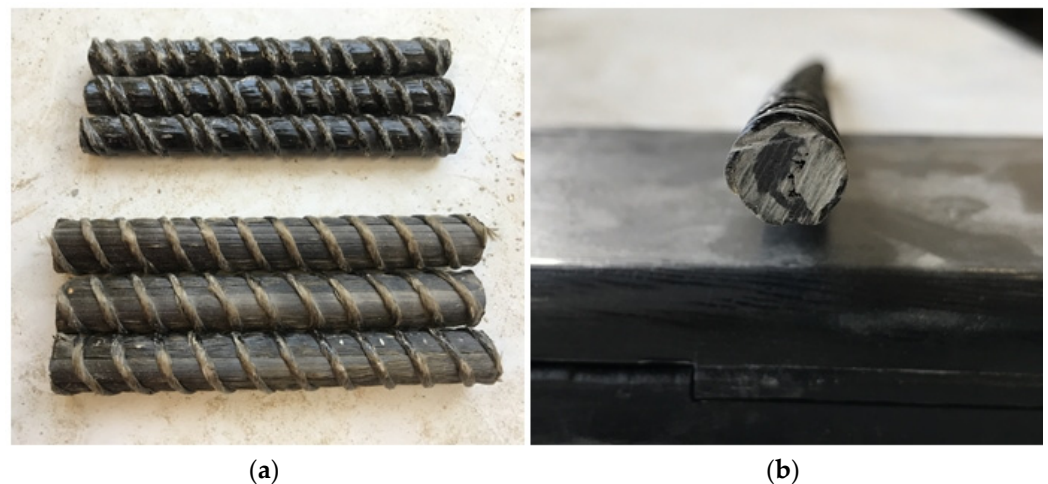
Figure 3. FRP bar imperfections: uneven coverage of epoxy resin on surface of bars (a) variable distance of the carbon core from the bar edges (b).
