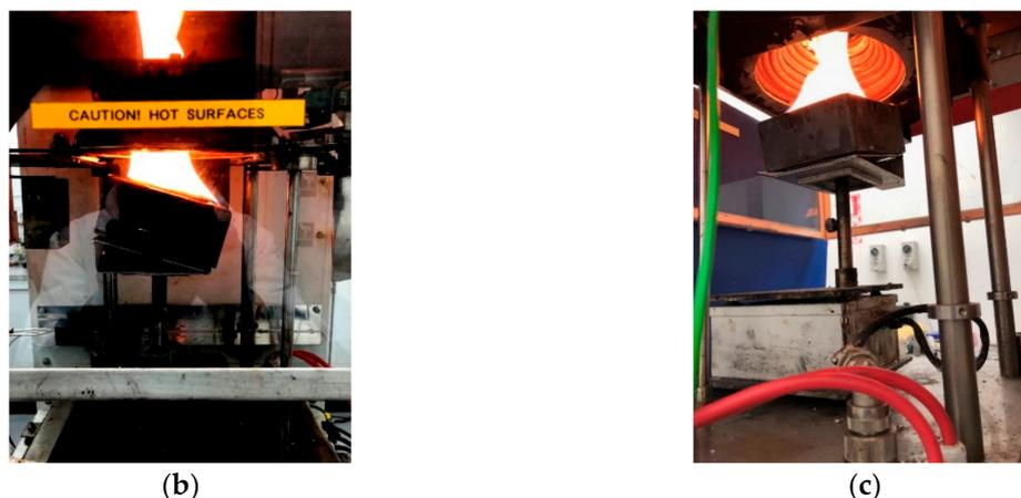
**Figure 1.** (a) Schematic 2D diagram of sample orientations relative to horizontal (i.e., heat flux normal) direction from the cone heater (b) Cone calorimeter experimental setup for an inclined sample orientation ( $15^\circ$  orientation)—front view, and (c) side view.
