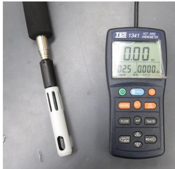
Figure 4. Hot wire anemometer.
