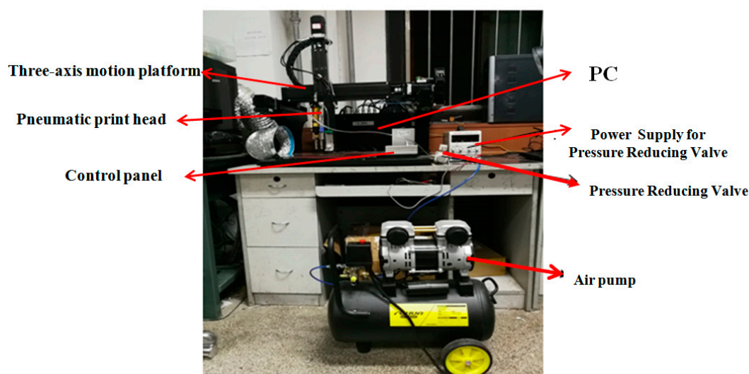
Figure S1. Experimental setup for the direct writing process.
