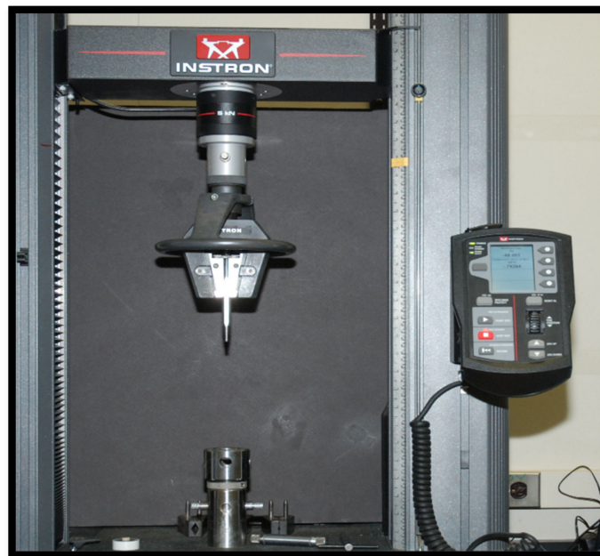
Figure 2. Testing equipment (Instron testing machine) used for denture fractures.
