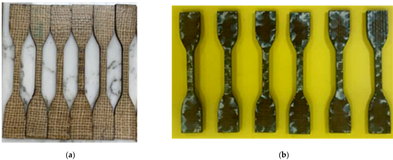
Figure 10. Tensile specimen (a) before and (b) after being immersed in distilled water for 28 days.
