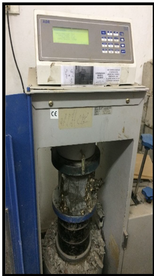
Figure 2. Concrete cubes under testing machine.
