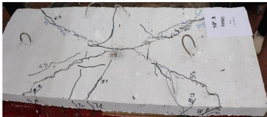
(c) Slab SP3
