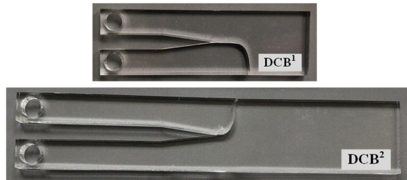
Figure 15. Broken blunt V-notched DCB 1 and DCB 2 specimens under mode I loading. \gamma = 15^\circ ; \rho = 0.125 mm.
