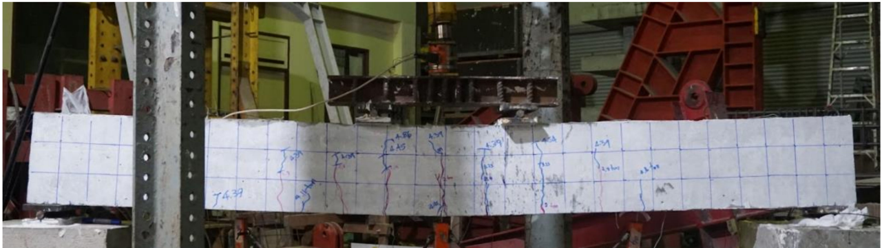
Figure 11. Final failure of control beam.
