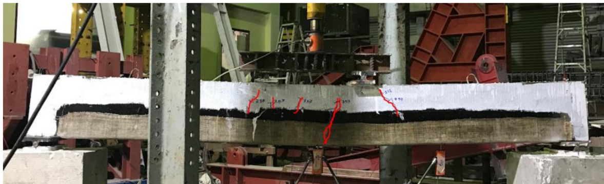
Figure 14. Final failure of specimen B-02.
