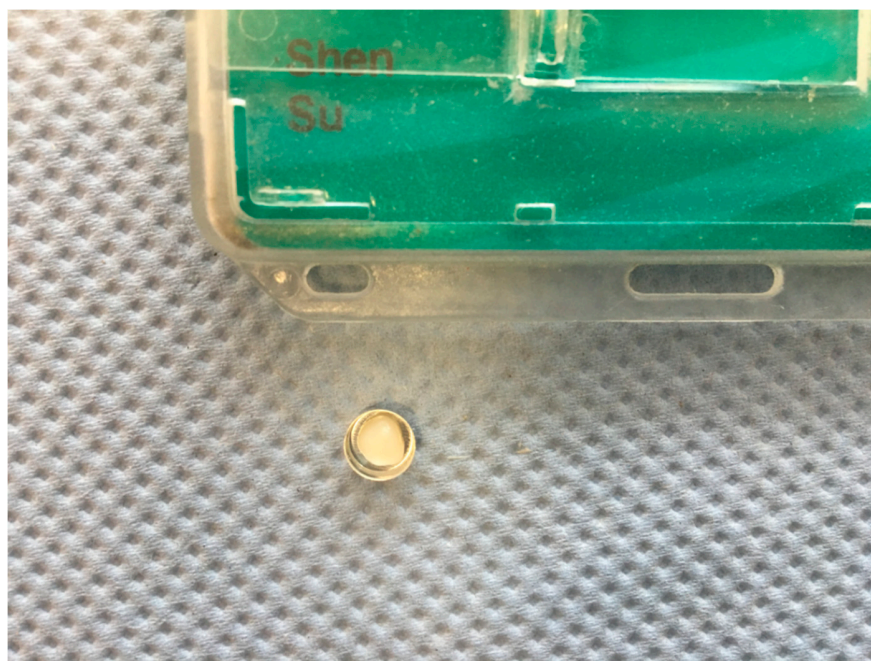
Figure S2. Prepared blend B0L0-55 in a TGA crucible with a Fraunhofer employee card in the background.
