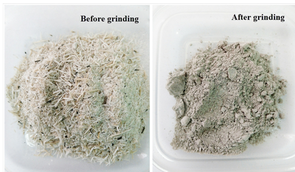
Figure 1. Images of RHA before (left) and after (right) grinding.
