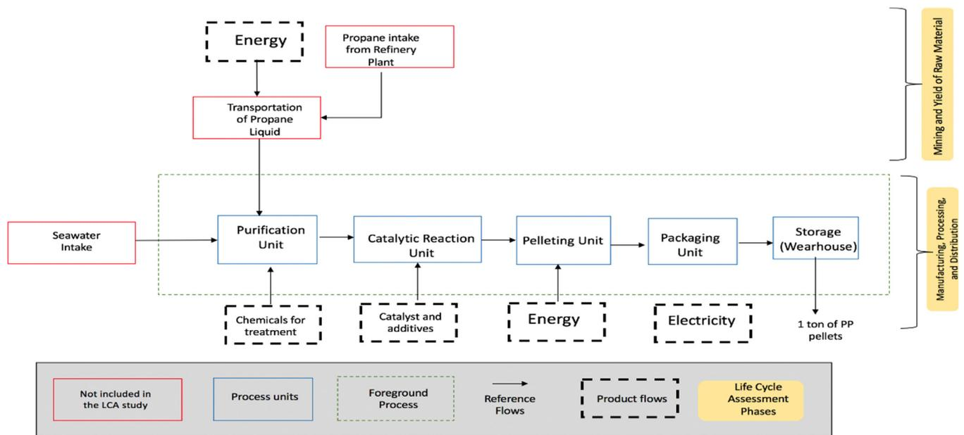
**Figure 3.** System boundaries for each unit in the PP manufacturing plant considered in this LCA study. The life cycle phases have been highlighted, while the construction of this plant, production of raw material, usage of PP, and the end-life scenarios for PP have been excluded from this LCA study.
