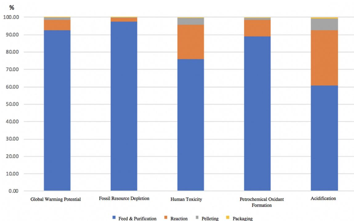
**Figure 4.** An overview for the impact assessment categories results for annual production of PP, representing the results for each process in the PP manufacturing plant, including the feed and purification phase.
