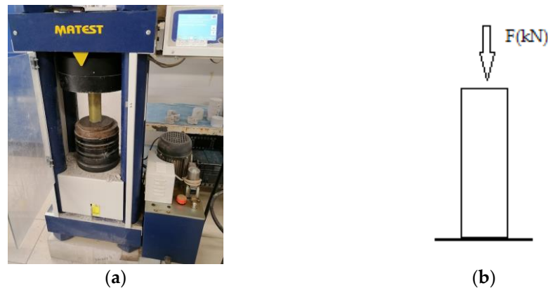
Figure 12. (a) MATEST TREVILOLO press of capacity 2000 kN during the compression tests; (b) representation of compression measurement.
