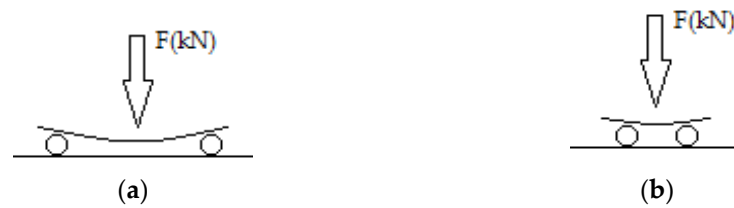
Figure 11. (a) Three-point scheme for the bending strength measurement; (b) three-point scheme for the shear strength measurement.
