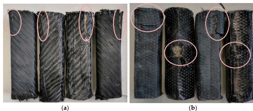
Figure 16. Compressed specimens reinforced with carbon fabric: (a) unidirectional fabric; (b) twill fabric.
