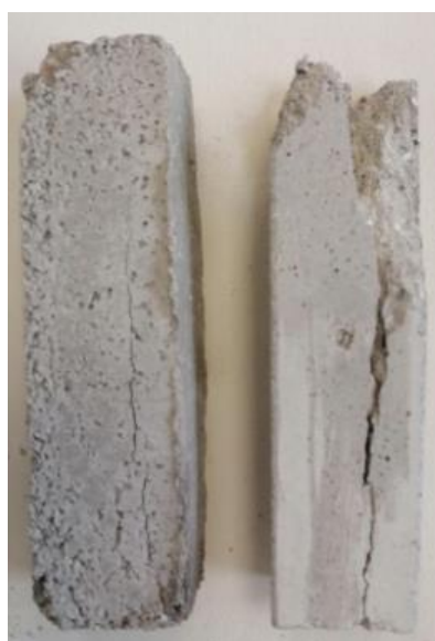
Figure 18. Compressed cement specimen without reinforcement (retrofitting).
