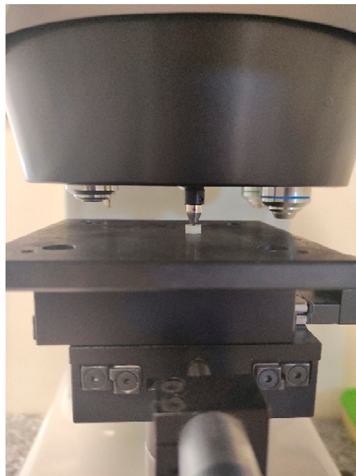
Figure 1. The sample during Vicker's hardness test.
