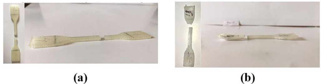
Figure 14. The tensile specimen (a) before, and (b) after the annealing process. Reprinted with permission from [82]. Copyright 2020, Emerald Publishing Limited.
