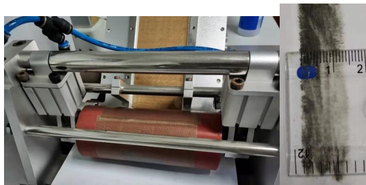
Figure 6. Measurement experiment of contact length of the flexible compactor.
