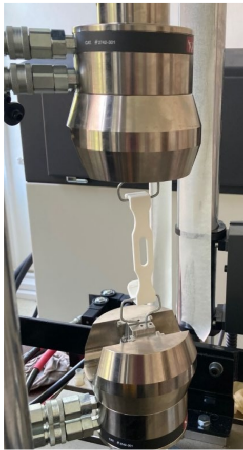
Figure 3. Experimental set-up for the testing of surgical retractors.
