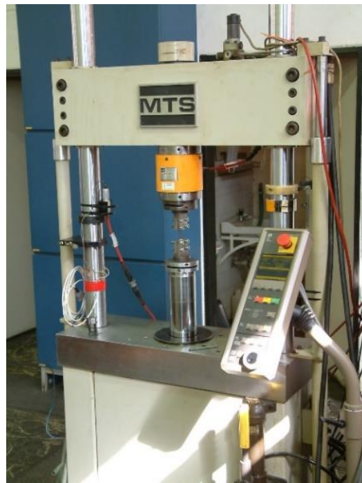
Figure 4. MTS tensile testing machine.
