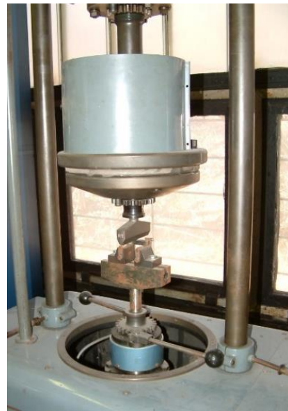
Figure 7. Three-point bending test machine.
