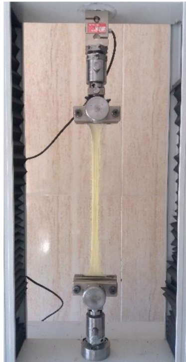
Figure 3. Tensile test of the fabric.
