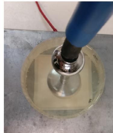
**Figure 6.** Experimental setup with a dielectric layer of epoxy resin and the electrode surrounded by epoxy resin too.
