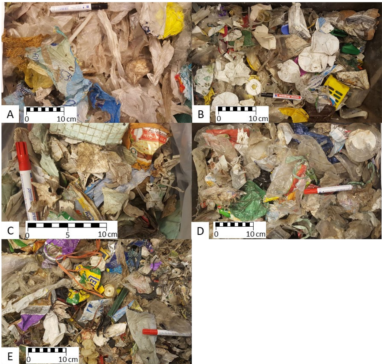
Figure A4. Exemplary photos of plastic types sorted with NIR: PE—A; PP—B; PET—C; PS—D; and others—E.
