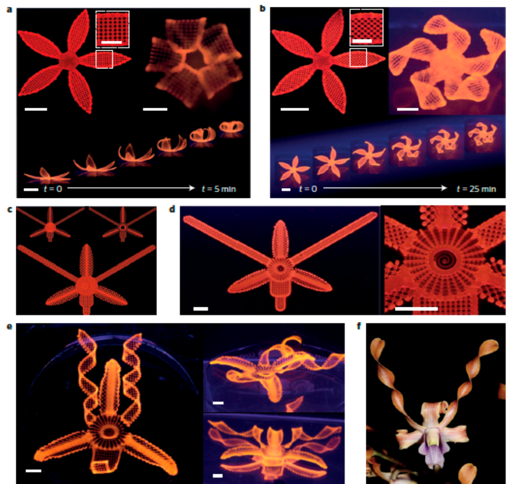
Figure 5. Complex flower morphologies generated by biomimetic 4D printing. (a,b) Simple flowers composed of 90^\circ/0^\circ (a) and 45^\circ/45^\circ (b) bilayers oriented with respect to the long axis of each petal, with time-lapse sequences of the flowers during the swelling process (bottom panel) (scale bars, 5 mm, inset = 2.5 mm). (c–f) Print path (c), printed structure (d) and resulting swollen structure (e) of a flower demonstrating a range of morphologies inspired by a native orchid, the Dendrobium helix (f). Based on the print path, this orchid architecture exhibits four different configurations: bending, twisting and ruing corolla surrounding the central funnel-like domain (scale bars, 5 mm). Reprinted by permission from [208] published by Springer Nature.
