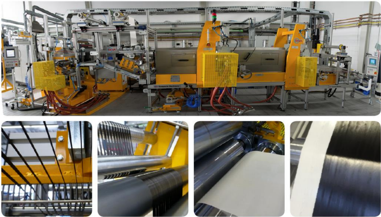
Figure 3. Above: Prepreg machinery at the Department of Polymer Engineering. Below, from left to right: sorting of single UD rovings, fiber pre-spreading unit, resin coating unit, and final produced prepreg, respectively.
