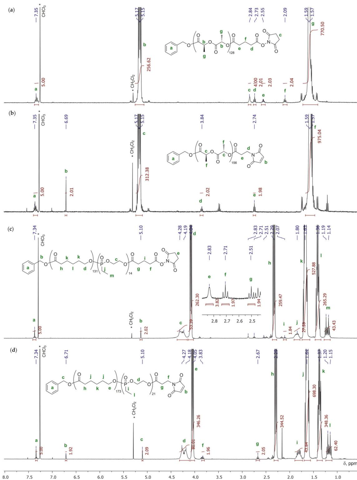
**Figure 1.**  $^1\text{H}$  NMR spectra of NHS- and MI-functionalized polymers (Table 1, Entries 7 (a), 8 (b), 11 (c), and 12 (d)). The signals of the protons of the fragments of functionalized polymers are marked as letters (bold and green) the solvent impurities are marked by asterisks (\*). 3.2. Functionalization by the Reaction of the Polymers with Acyl Chloride 1.
