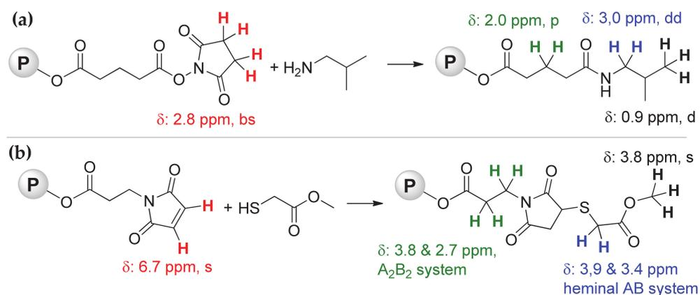
**Scheme 3.** Reactions of NHS- and MI-functionalized polymers with model amine and thiol,  $^1H$  NMR criteria of the completion of the processes for NHS- and MI-terminated polymers, (a) and (b), respectively.
