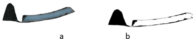
Figure 2. Scanned image of the melt cross section: (a) raw image, (b) after transformation to black and white.
