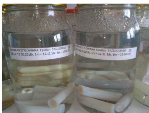
Figure 3. The examples of two glass vessels with E57/Z-1/10:1 epoxy compound samples immersed in rainwater and tap water.
