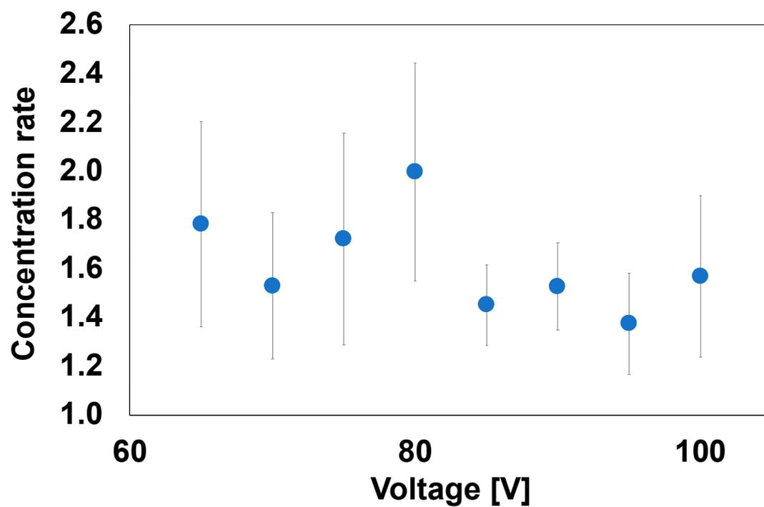
**Figure S4.** Concentration of negatively charged nanoparticles in a nanoparticle concentrator with a branched channel at constant flow rate ( $4 \mu\text{L}/\text{min}$ ;  $n = 5$ ).
