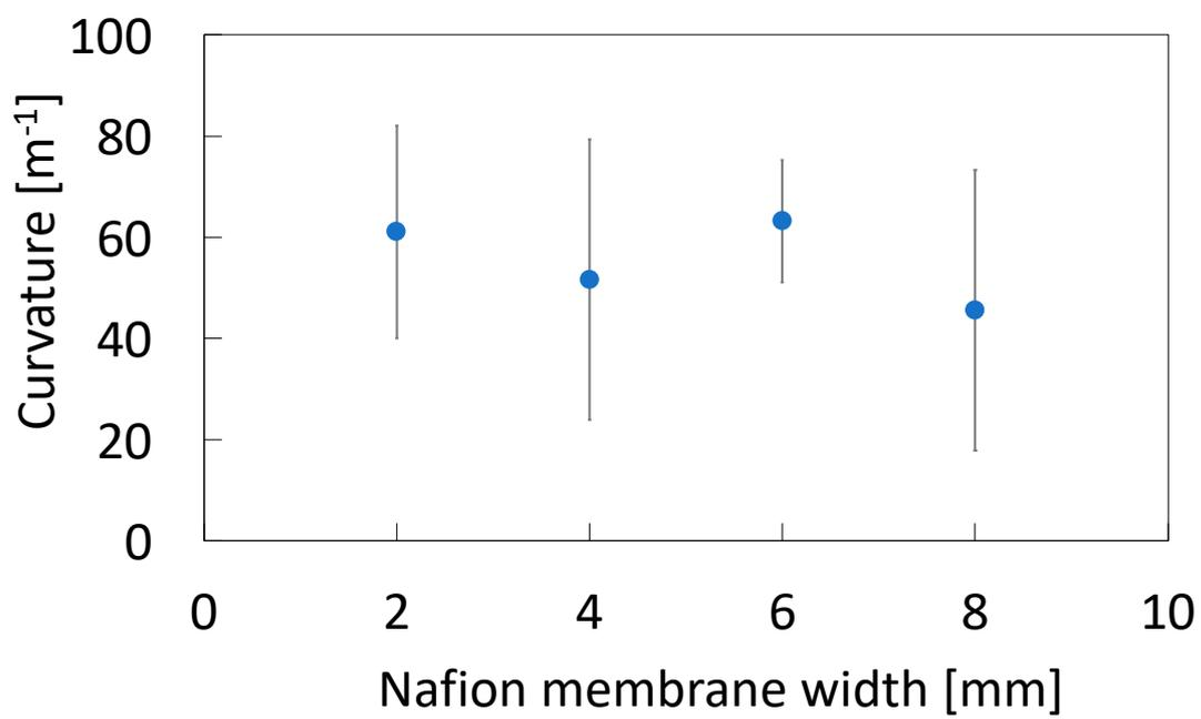
**Figure S1.** Relationship between Nafion membrane width and curvature at a constant heating temperature (25°C) (n = 5).
