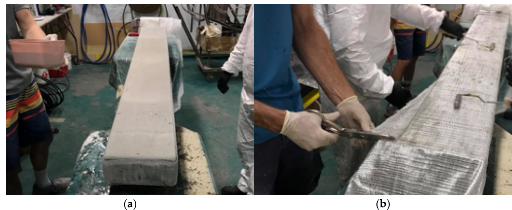
Figure 2. Manufacturing process. (a) Prefabricated PU foam core. (b) Applying GFRP fabrics on PU core.
