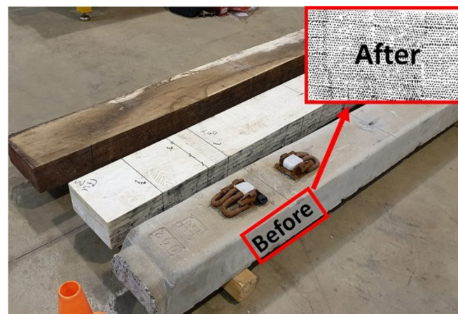
Figure 6. Sleeper samples showing applied speckle pattern.
