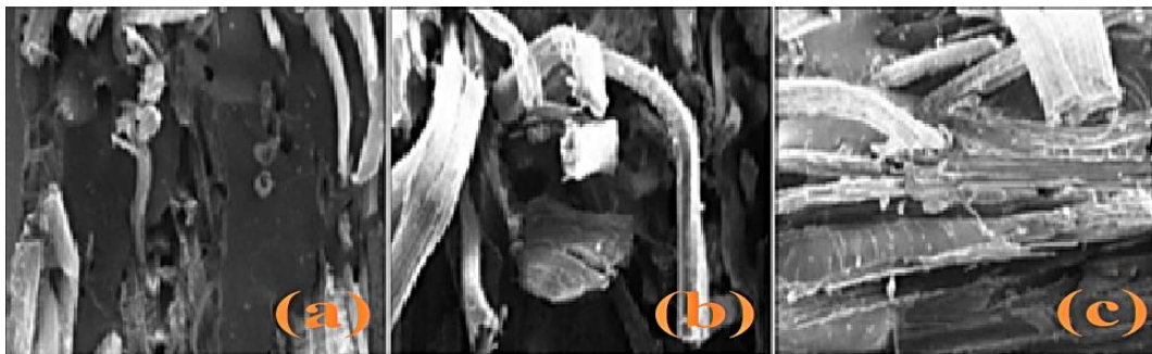
Figure 17. (a–c) SEM images of the flexural fractured specimen at different fiber loading, (a) 25 wt. %, (b) 35 wt. %, and (c) 45 wt. % of pineapple-reinforced polyester composites. Reprinted with the permission from Reference [95]. Copyright 2019 Elsevier.
